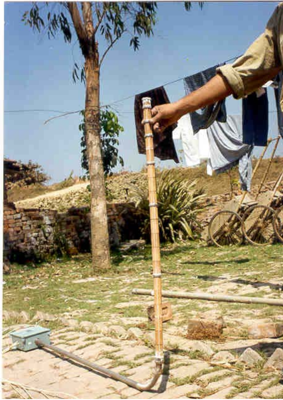
Fig. 3. A Ground thermocouple assembly
